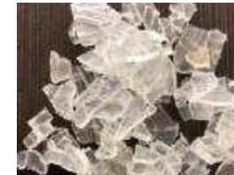
Glass from broken solar panel
