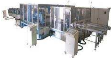
Provision of solar panel disassembly equipment
