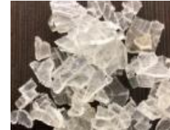
Glass from broken solar panel
